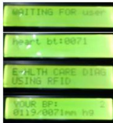
**Fig.6.** Sensor Output broadcasting heart rate & BP in the LCD Module
