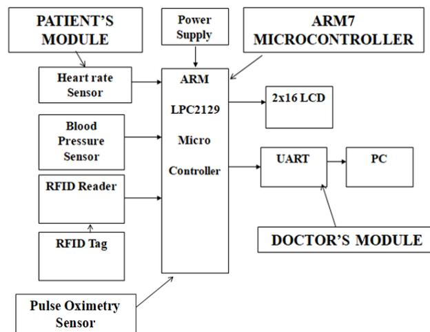
Fig.1. Block diagram of the proposed healthcare diagnosis System
