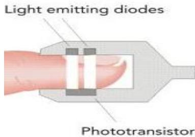
**Fig.3.**pulse oxymetry sensor
