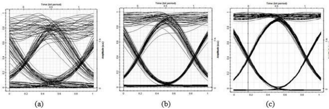
Figure 4: Eye Diagrams for Different Input Power Values (a) 0 dBm, (b) -10dBm, (c) -20 dBm
