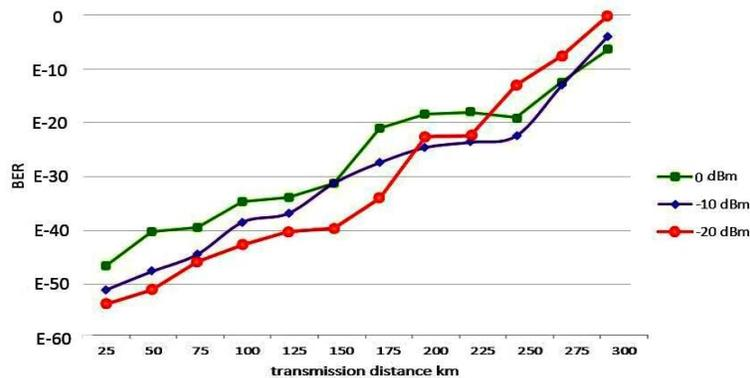
Figure 3: BER vs. Fiber Length
