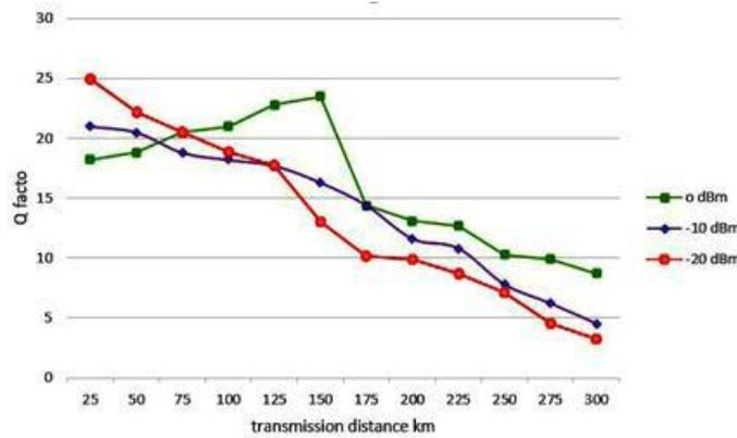
Figure 2: Q Factor vs. Fiber length
