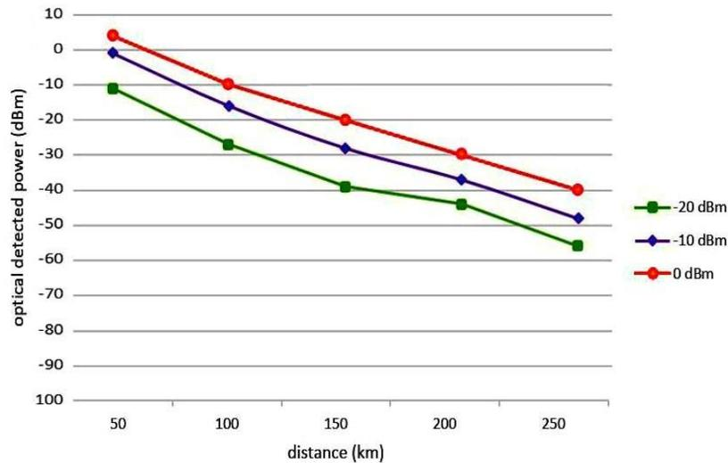
Figure 6: Received Power vs. Distance
