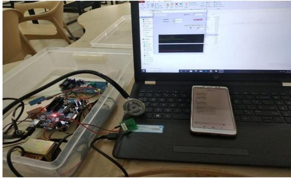
**Fig.3.**Experimental setup of fetal heart rate monitoring and uterus contraction.
