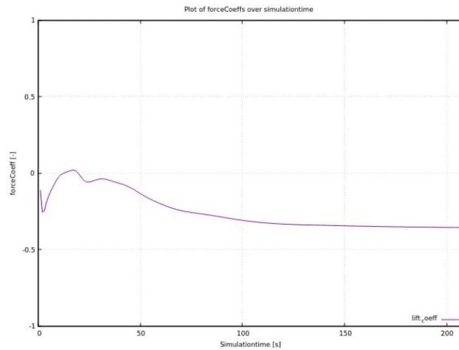
**Fig 5. Simulation graph coefficient of lift with respect to no angle of attack of aircraft at cruise altitude.**
