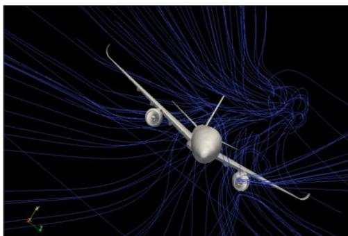
Fig 2. Streamline and turbulent airflow around the aircraft.
