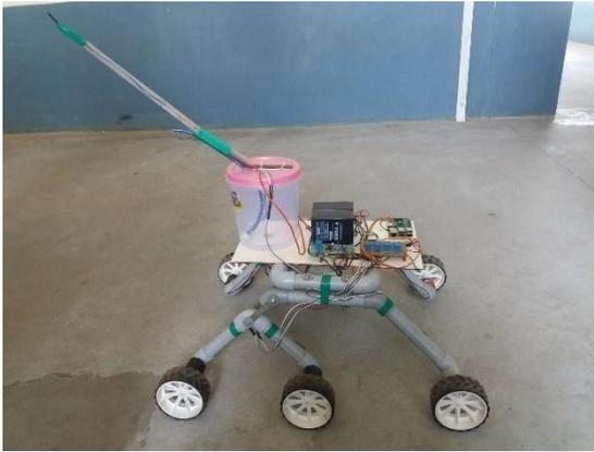
**Figure 5. The fire extinguishing robot**
