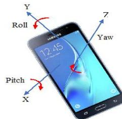
**Fig. 4 Direction of acceleration signals**
