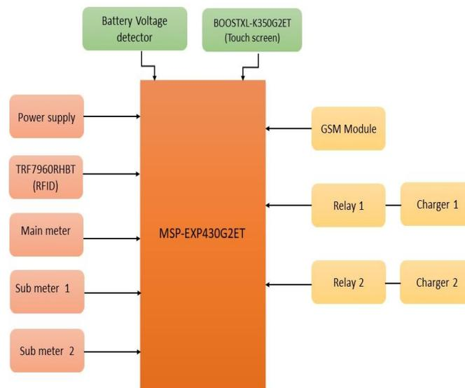
**Fig 4:** Block Diagram of E-metering.
