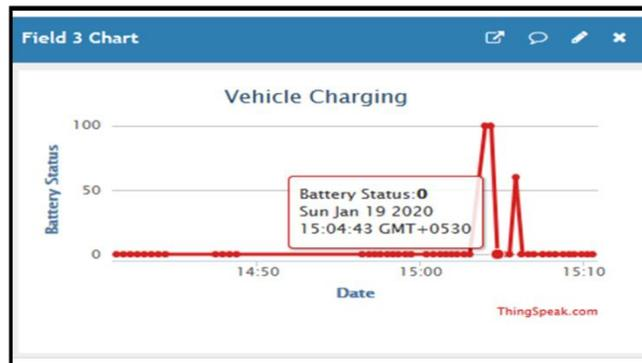
**Fig. 12:** Battery status when connect for charging with respect to time
