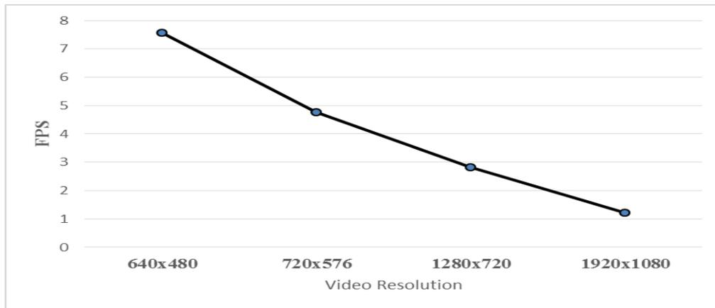
**Fig. 10:** Plot of video resolution vs. FPS for the proposed system
