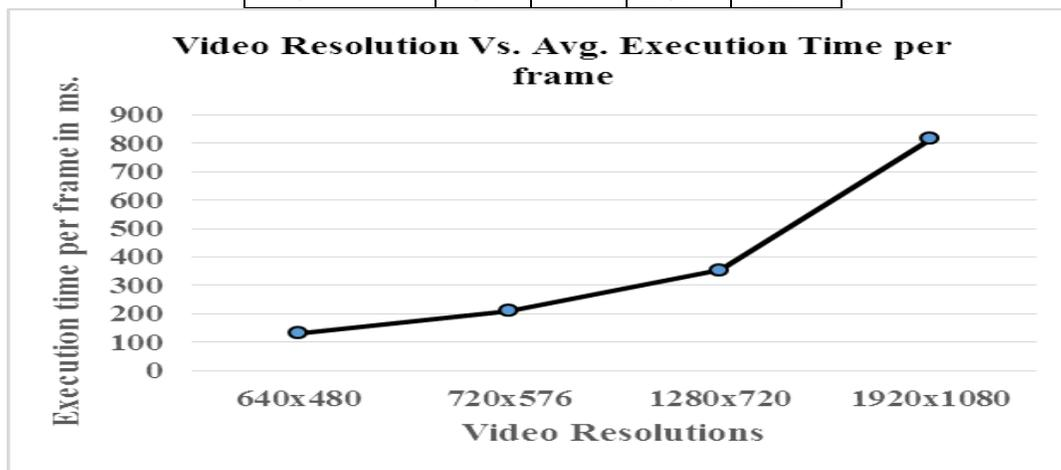
Fig. 9: Plot of video resolution vs. execution time per frame in millisecond for the proposed system
