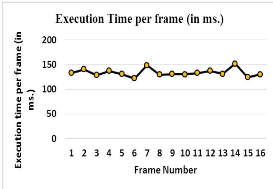
**Fig. : 4** Plot of execution time per frame (in ms.) vs. frame number for 640x480 resolution video
