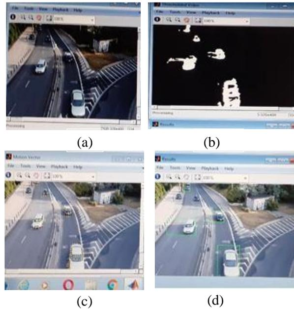
**Fig. 3:** Different Images for the frames a) Original Image b) Threshold Image c) Image with motion vector d) Image with the object detected
