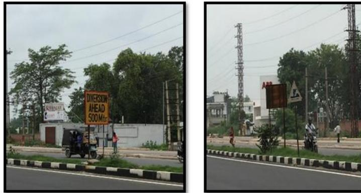
**Figure 5** Sign boards without retro-refractory background& Men at Work is faded not visible clearly
