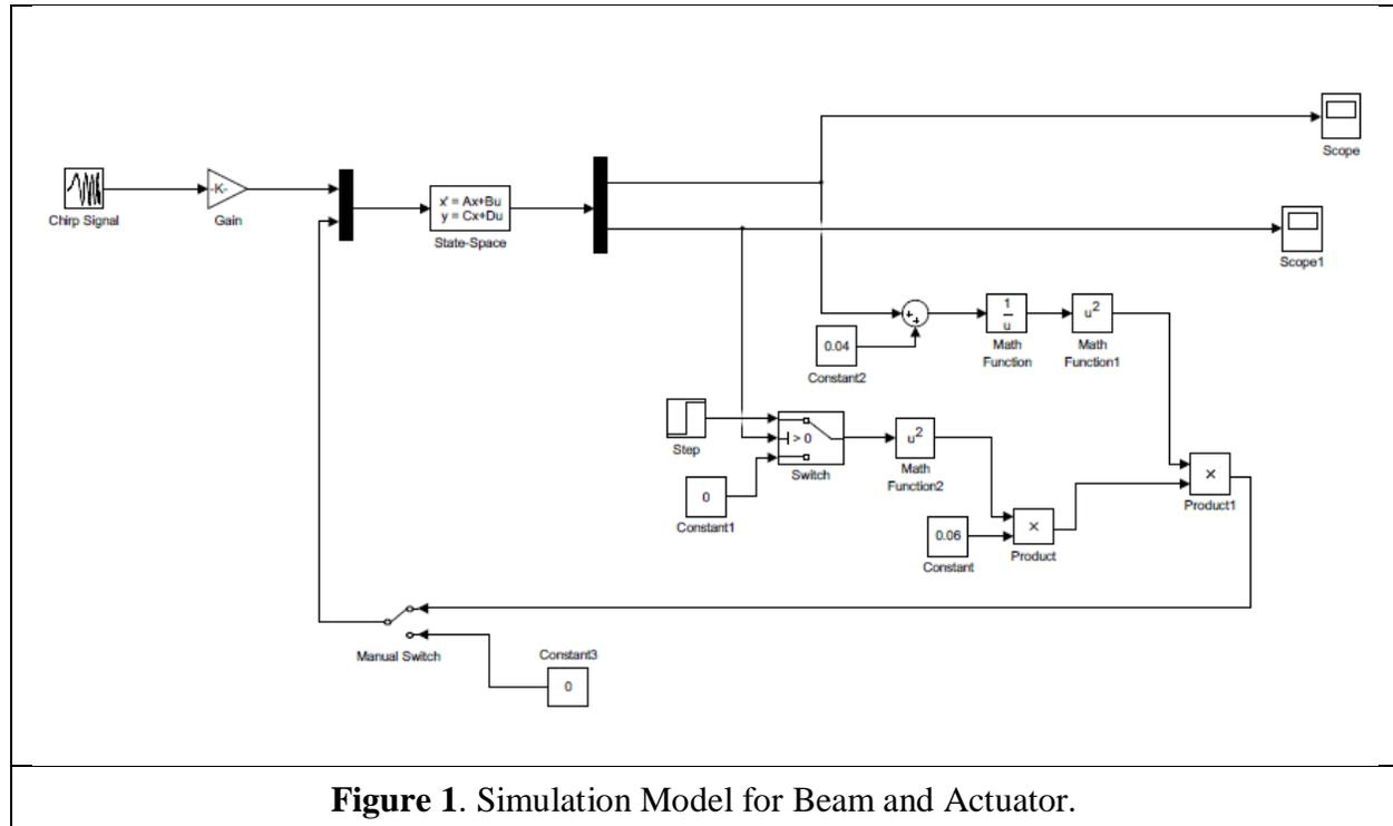
**Figure 1.** Simulation Model for Beam and Actuator.
