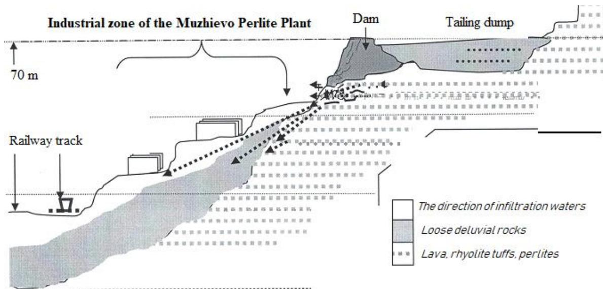
Figure 2 – Tailings dump position relative to other facilities
