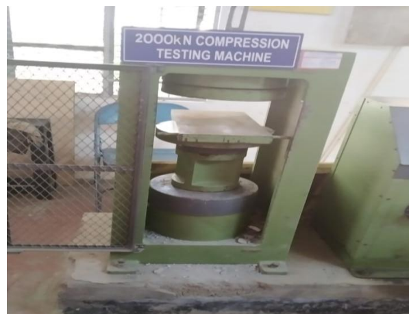
Figure 2.5: Compressive testing machine
