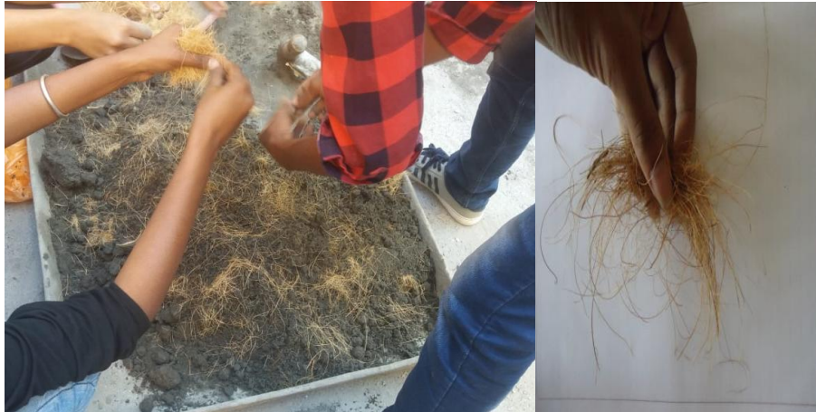
Figure 2.4: Mixing of coir fibers with mortar
