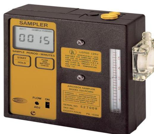
Fig. Personal Air Sampler
