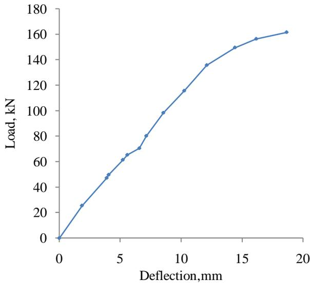
Fig. 5 Normalised pre-peak load-deflection curve of PFRC specimen
