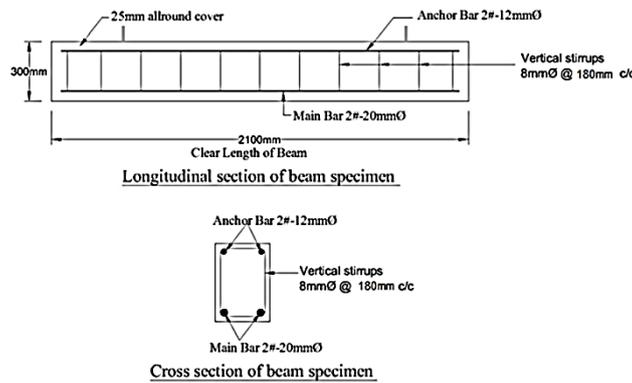
Fig.3 Reinforcement details of RC beam specimen
