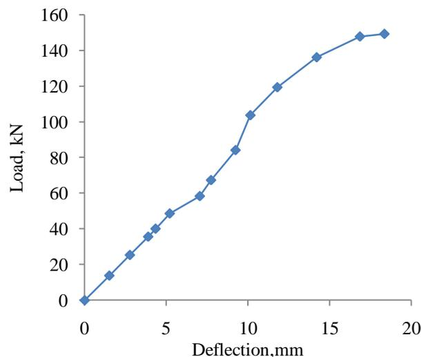
Fig. 4 Normalised pre-peak load-deflection curve of CC specimen
