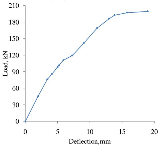
Fig.6 Normalised pre-peak load-deflection curve of SFRC specimen
