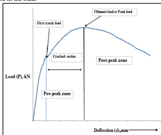
Fig 1 Typical load deflection curve
