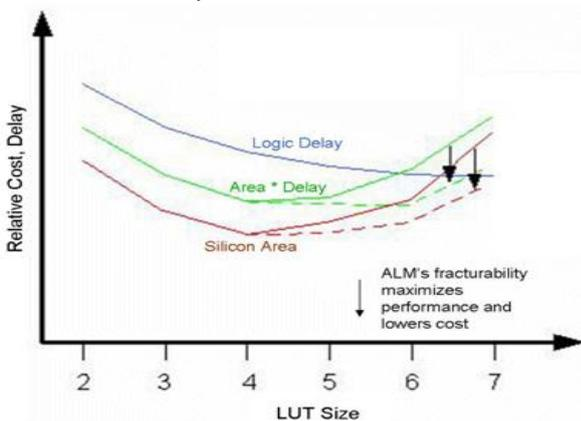
Fig. 7. Cost-logic delay tradeoff with varying LUT sizes
