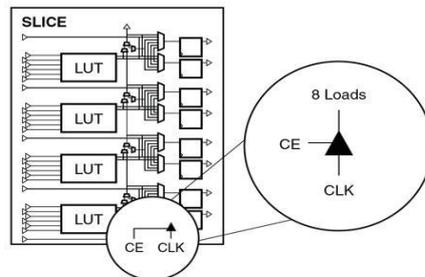
Fig. 4. LUT clock gating buffer
