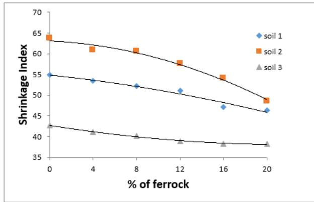
Fig 7 Correlation of Shrinkage Index with different percentages of Ferrock replacement by weight
