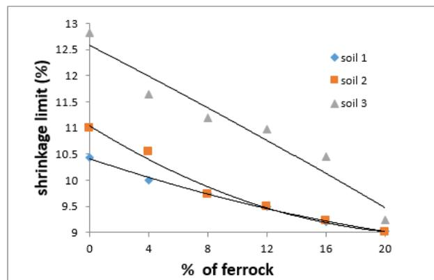
**Fig 6 Correlation of Shrinkage Limit with different percentage of ferrock replacement by weight**
