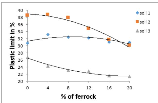
**Fig 4 Correlation of Plastic Limit with different percentages of Ferrock replacement by weight**
