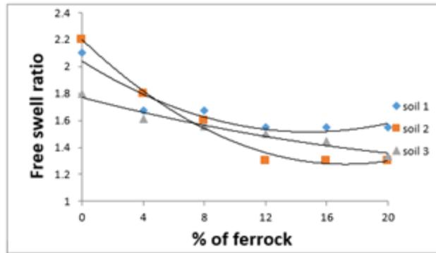
**Fig 1 Correlation of free swell ration with different percentage of ferrock replacement by weight**
