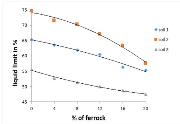
**Fig 3 Correlation of Liquid Limit with different percentages of Ferrock replacement by weight**
