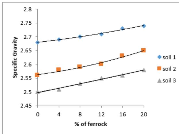
**Fig 2 Correlation of Specific Gravity with different percentage of Ferrock**
