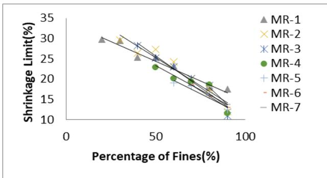
**Fig. 7 (a)** Correlation of shrinkage limit with percent fines for different compaction energy levels for MR-1 through MR-7.
