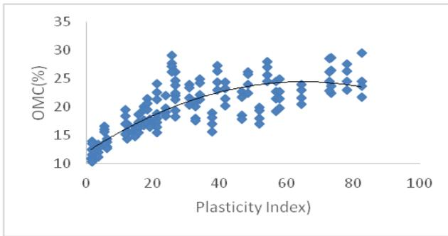
**Fig. 10 (a)** Correlation between OMC and  $I_p$  for different energy levels for MR-1 through MR-7.
