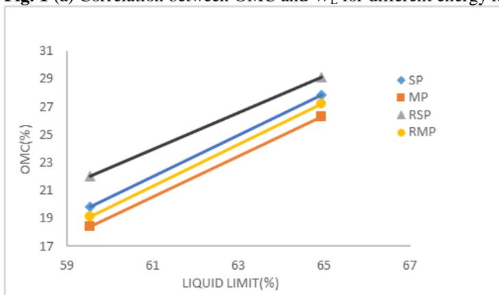
**Fig. 1 (b)** Correlation between OMC and W<sub>L</sub> for different energy levels for MR-7.
