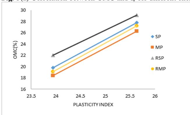
**Fig. 5(b)** Correlation between OMC and  $I_p$  for different energy levels for MR-7.
