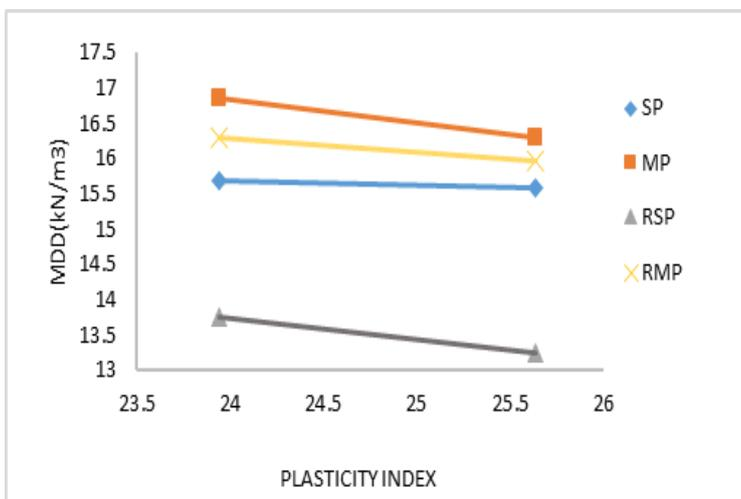
**Fig. 6(b)** Correlation between MDD and I<sub>p</sub> for different energy levels for MR-7.
