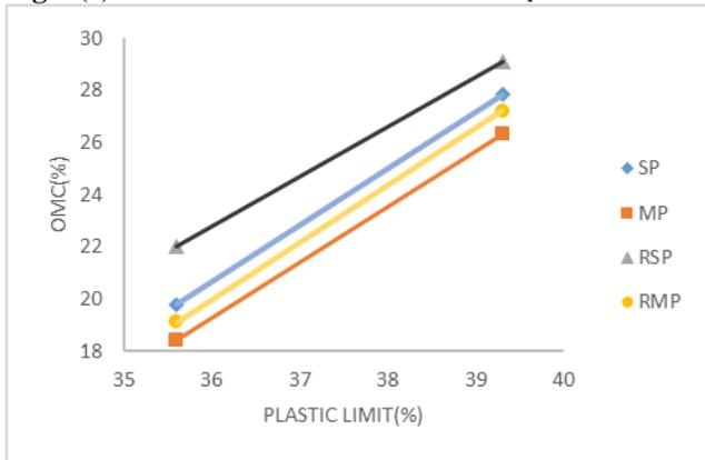
**Fig. 3(b)** Correlation between OMC and  $W_p$  for different energy levels for MR-7.
