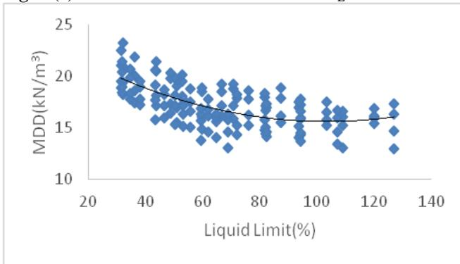
**Fig. 8 (b)** Correlation between MDD and  $W_L$  for different energy levels for MR-1 through MR-7.
