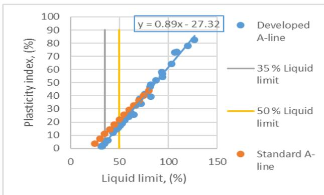
**Fig. 7 (b)** New plasticity chart developed for mix proportions.
