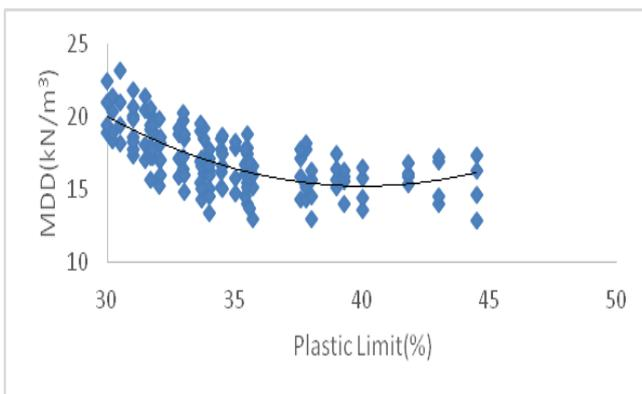
**Fig. 9 (b)** Correlation between MDD and  $W_P$  for different energy levels for MR-1 through MR-7.
