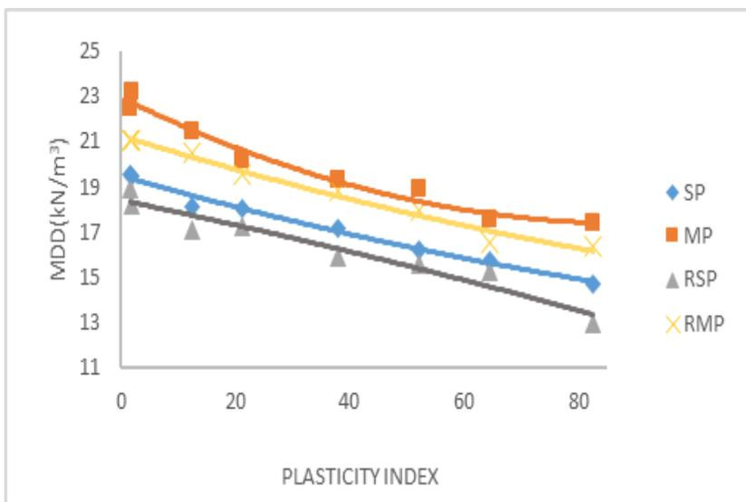
**Fig. 6(a)** Correlation between MDD and I<sub>p</sub> for different energy levels for MR-1.
