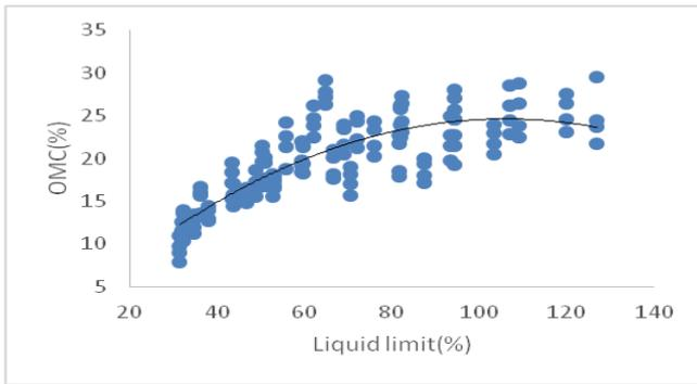
**Fig. 8 (a)** Correlation between OMC and  $W_L$  for different energy levels for MR-1 through MR-7.
