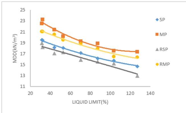
**Fig. 2(a)** Correlation between MDD and W<sub>L</sub> for different energy levels for MR-1.
