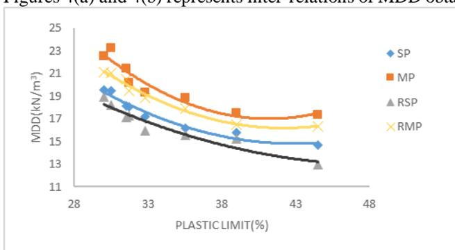
**Fig. 4(a)** Correlation between MDD and  $W_p$  for different energy levels for MR-1.
