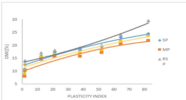
**Fig. 5(a)** Correlation between OMC and  $I_p$  for different energy levels for MR-1.
