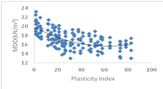
**Fig. 10 (b)** Correlation between MDD and  $I_p$  for different energy levels of samples of Table-1.
