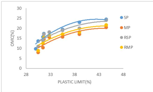
**Fig. 3(a)** Correlation between OMC and  $W_p$  for different energy levels for MR-1.
