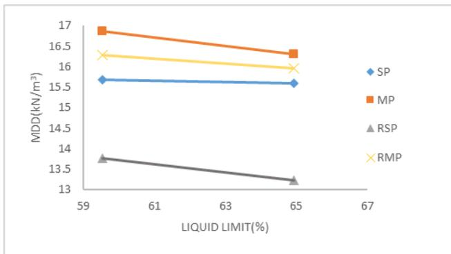
**Fig. 2(b)** Correlation between MDD and W<sub>L</sub> for different energy levels for MR-7.
