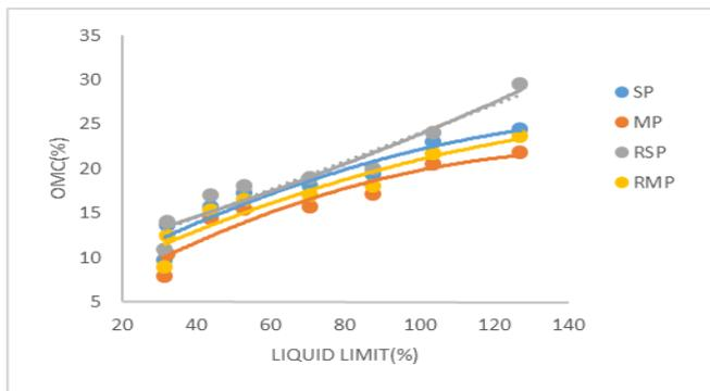
**Fig. 1 (a)** Correlation between OMC and W<sub>L</sub> for different energy levels for MR-1.
