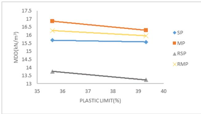
**Fig. 4(b)** Correlation between MDD and  $W_p$  for different energy levels for MR-7.
