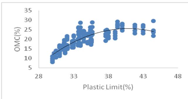
**Fig. 9 (a)** Correlation between OMC and  $W_P$  for different energy levels for MR-1 through MR-7.
