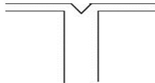
**Fig.4.** Mitered 'T' bend.
