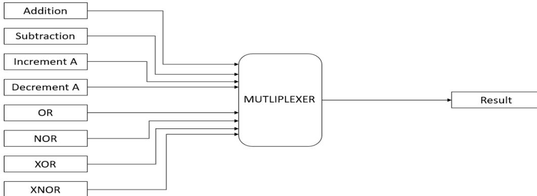
**Figure 3:** Block Diagram of ALU using irreversible gates
