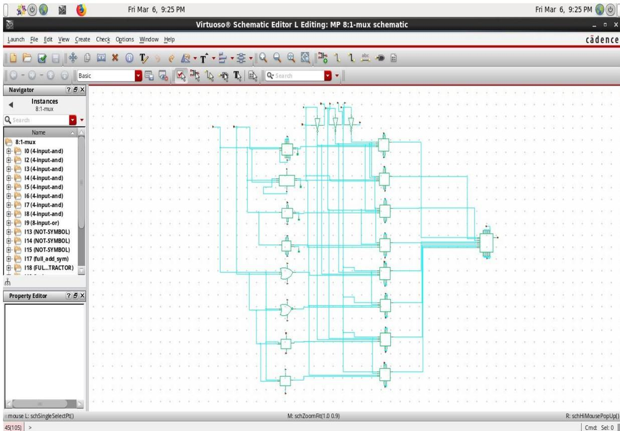
**Figure 4:** Schematic of ALU using irreversible gates
