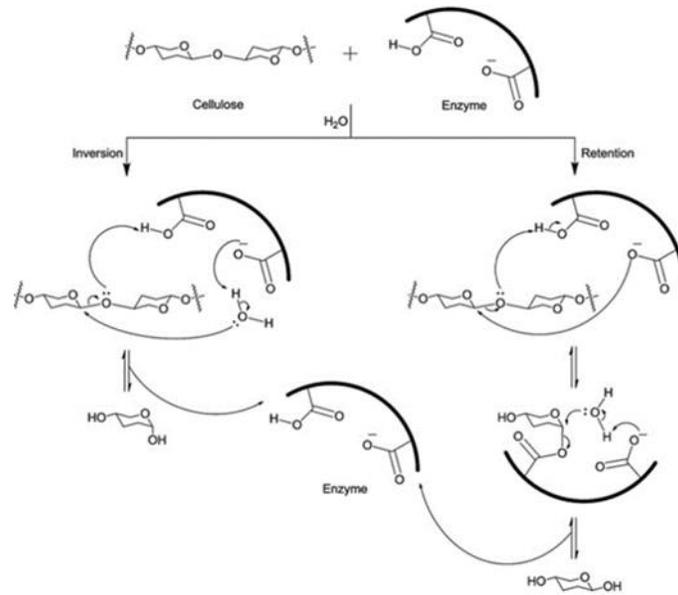
**Fig. 2** Enzymatic hydrolysis chemical process
