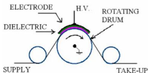
**Fig.3** A schematic of the continuous online processing of DBD plasma treatment of textile substrates
