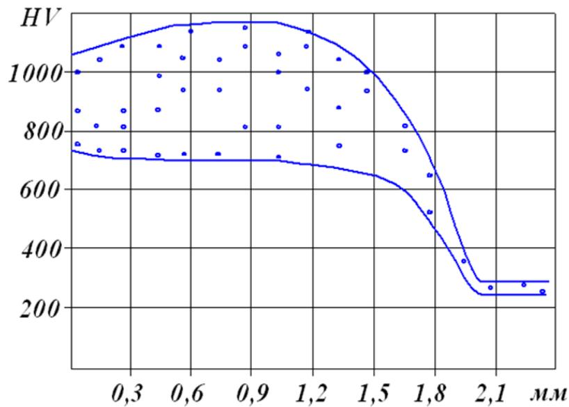
FIGURE 3: Distribution of hardness over the cross-section of a hard-alloy coating MLC - solid working element " ПГ-C27 - ЛКC 65ГЛ "
