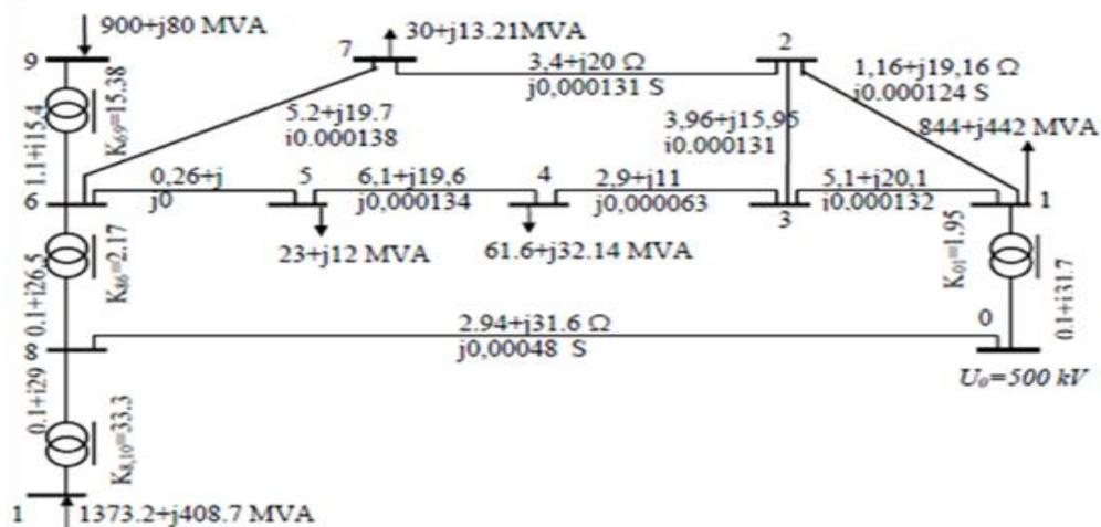
FIGURE 2: Scheme of the electrical network
