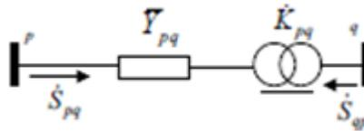
FIGURE 1: Representation of the transformer branch while optimization of its ratio.
