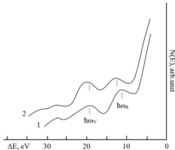
FIGURE: 1. Spectra of the characteristic energy loss of electrons for 1 -  $\text{GaP}(111)$ ; 2 -  $\text{GaP}(111)$  with a  $\text{Ga}_{0.6}\text{Al}_{0.4}\text{P}$  film.
