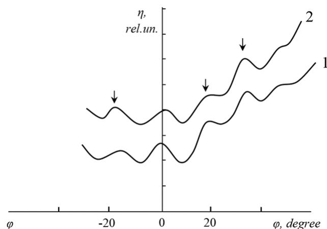
FIGURE: 2. Dependence of  $\eta$  on the angle of incidence  $\varphi$  of the primary electron beam for: 1 - GaP(111) single crystal, 2 - GaP(111) with a  $\text{Ga}_{0.6}\text{Al}_{0.4}\text{P}$  film 35–40 Å thick
