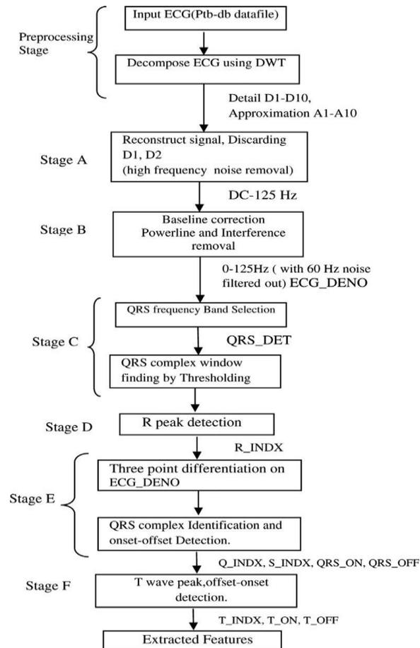
Fig. 3. Block schematic of the processing stages.
