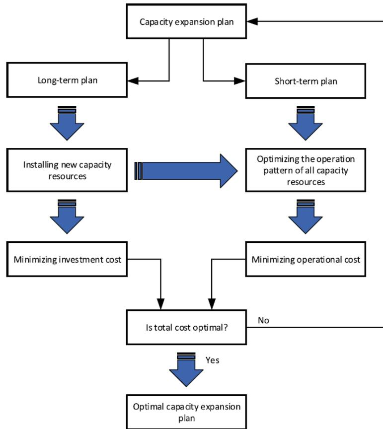
**Figure 2: Capacity Expansion Plan Flowchart for Long Term and Short Term.**
