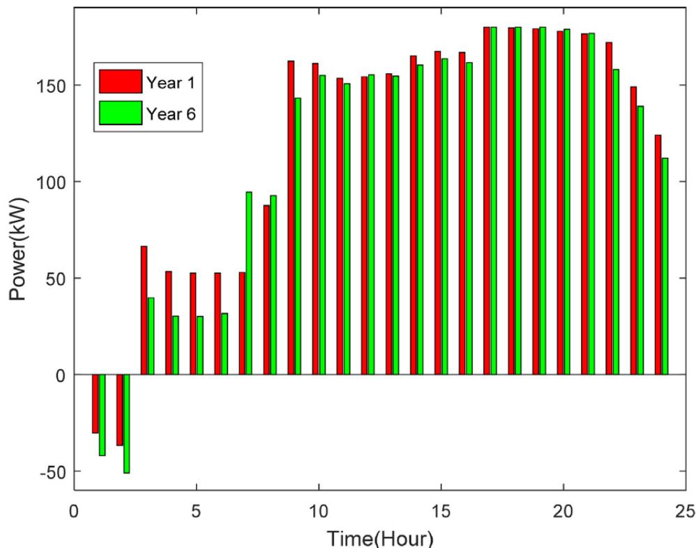
**Figure 4: Exchanged power between microgrid and upstream network in different years.**
