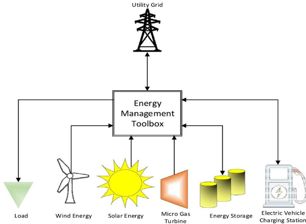
Figure 1: Proposed Structure of Microgrid.
