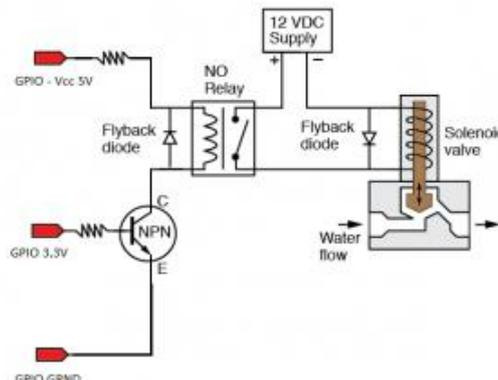
**Figure 3. Circuit diagram of the wiring in solenoid valve**
