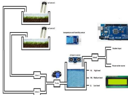
**Fig. 4 Design of plant Watering System.**
