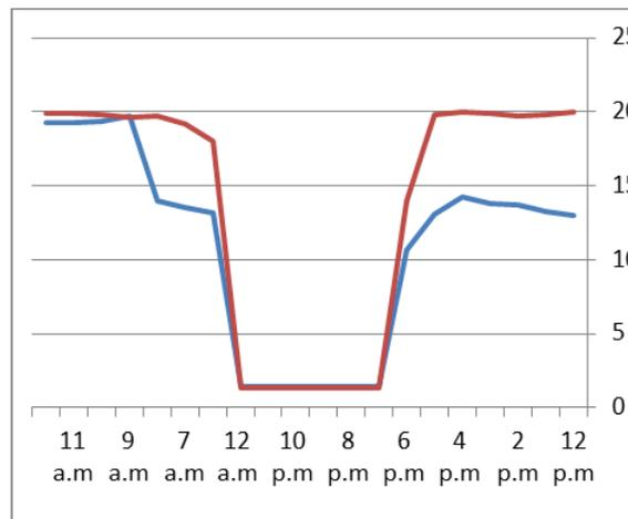
**Fig 3. The output voltage comparison of the proposed dual axis solar tracker (red color) with static solar panel (blue color). The Y-axis represents the output voltage of the solar panel and X-axis represents the time.**
