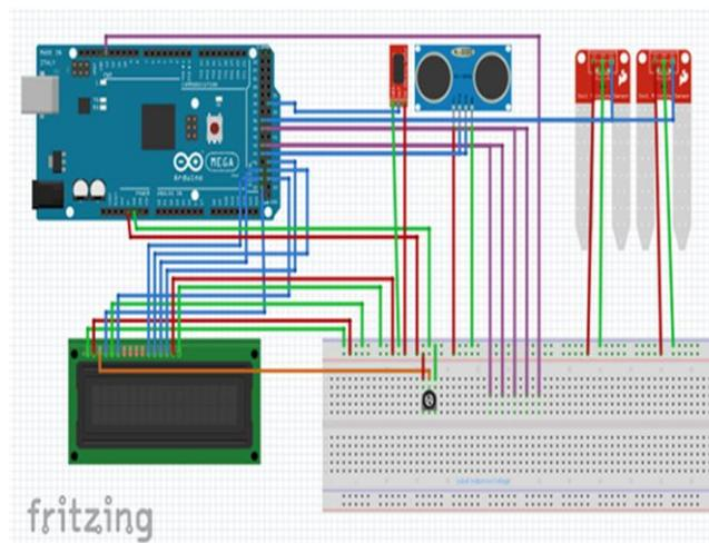
**Fig 5. Connection diagram of smart garden system.**
