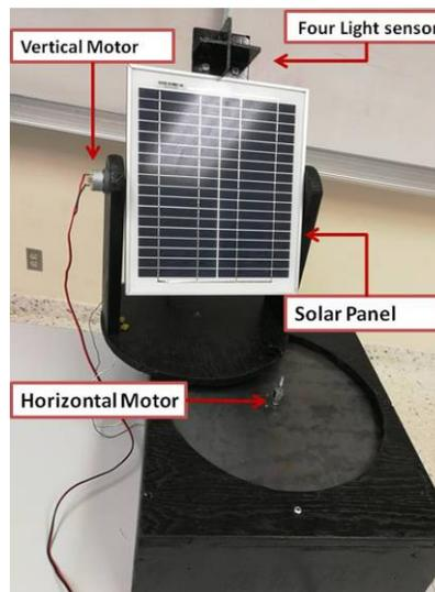
**Fig. 1. Prototype of Dual Axis solar tracker system**
