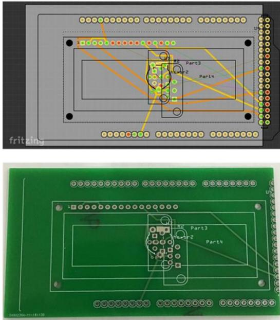
**Fig. 7. PCB design and fabrication of smart garden system**
