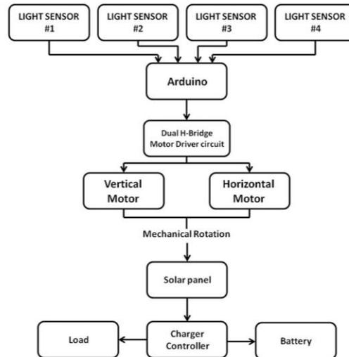
**Block Diagram of Dual Axis solar tracker system**
