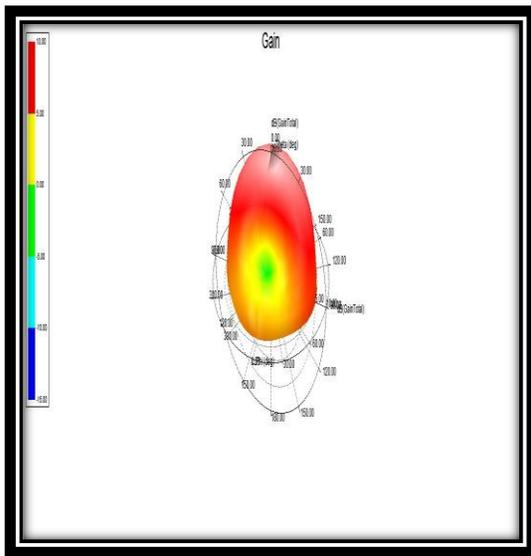
**Figure. 5. Gain of the antenna with co-axial feed**
