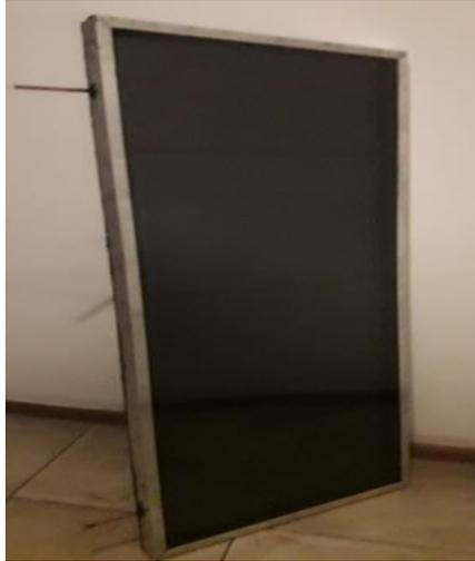
Figure 4- Flat solar collector mockup
