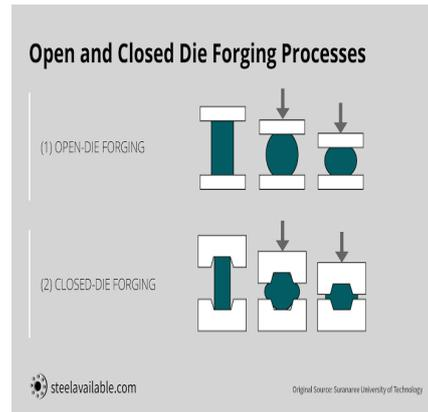
Significant sorts of forging process
