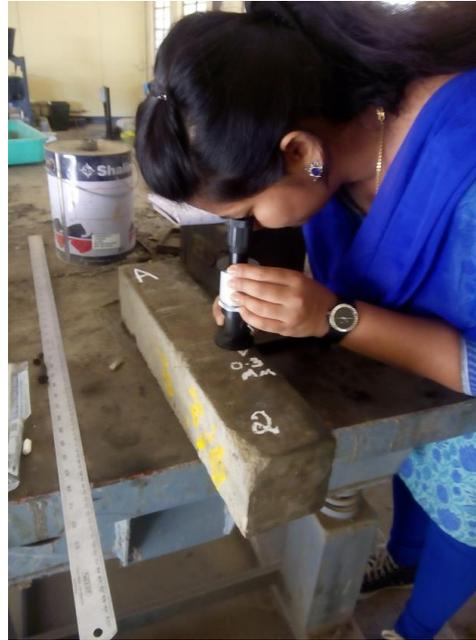
**Fig. 9 Crack width measuring using micrometer**
