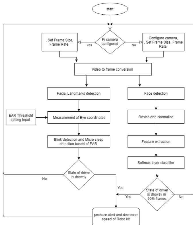
Fig.1. Design of the proposed hybrid model
