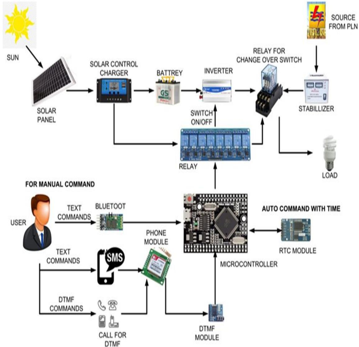
Figure 1. Chart of Smarthome Installation Implementation Based on Energy management
