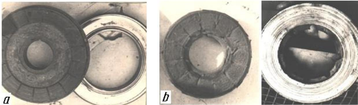
**Fig. 1. Wear of the thrust bearing of the electric pump ESW 10-120-60 (a - initial stage, b - ultimate state)**
