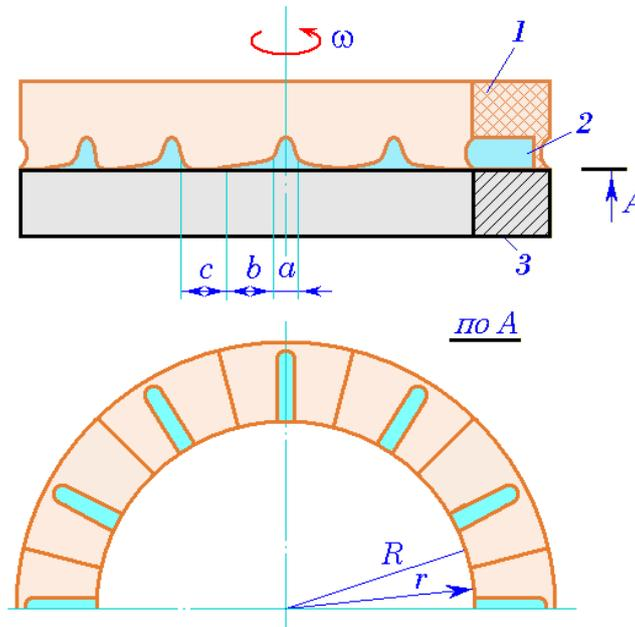
**Fig. 3. The calculation model of the end pair of sliding friction of the pump unit: 1 - heel; 2 - water; 3 – tilted pad unit.**
