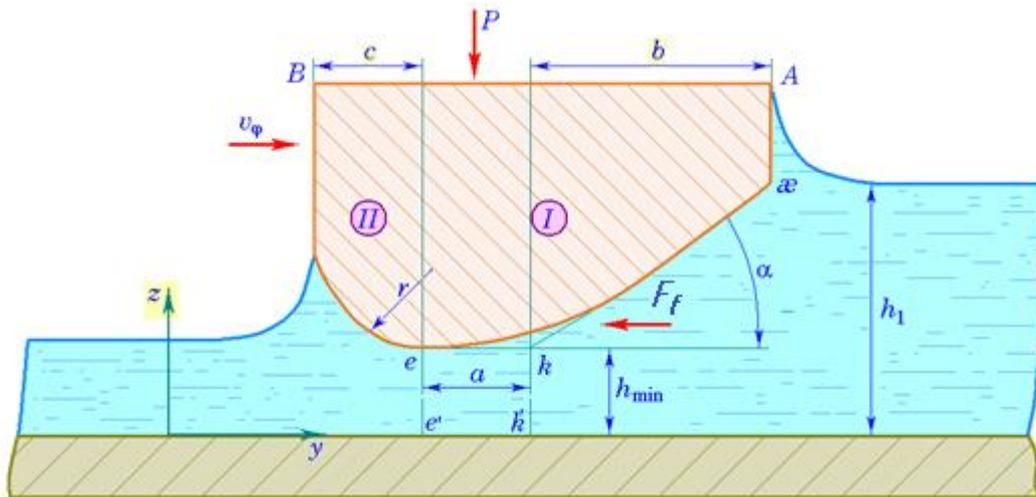
**Fig. 4. Sectorial model of the heel lift using a hydraulic wedge.**
