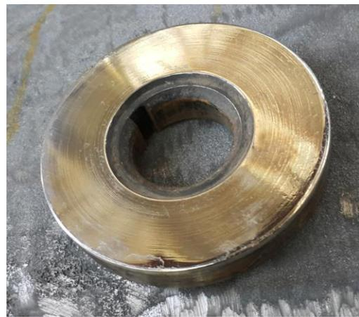
**Fig. 6. The tilted pad unit and the heel of the ECW 10-160-30 pump after the test.**
