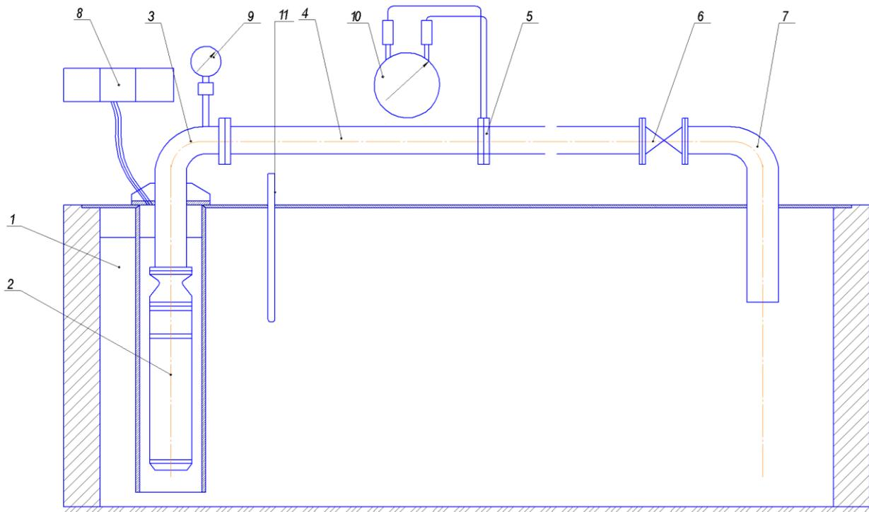
**Fig. 5. Test bench for pumps of ECW type: 1 - capacity, 2 - tested unit, 3 - connecting pipe, 4 - dimensional section, 5 - stone diaphragm, 6 - valve, 7 - discharge pipe, 8 - set K-505 , 9 - pressure gauge, 10 - differential pressure gauge-flow meter, 11 - thermometer.**
