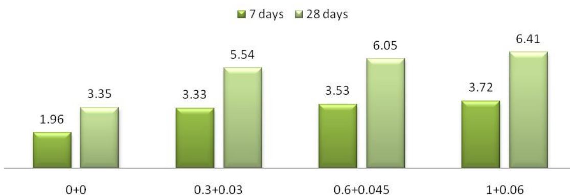
Fig. 8: Split Tensile Strength of concrete replacing the cement with Nano Silica & MWCNT
