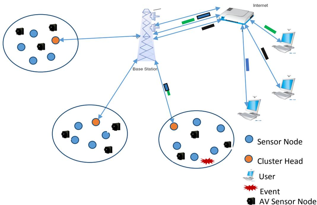
**Figure 1. Architecture of wireless multimedia sensor networks**
