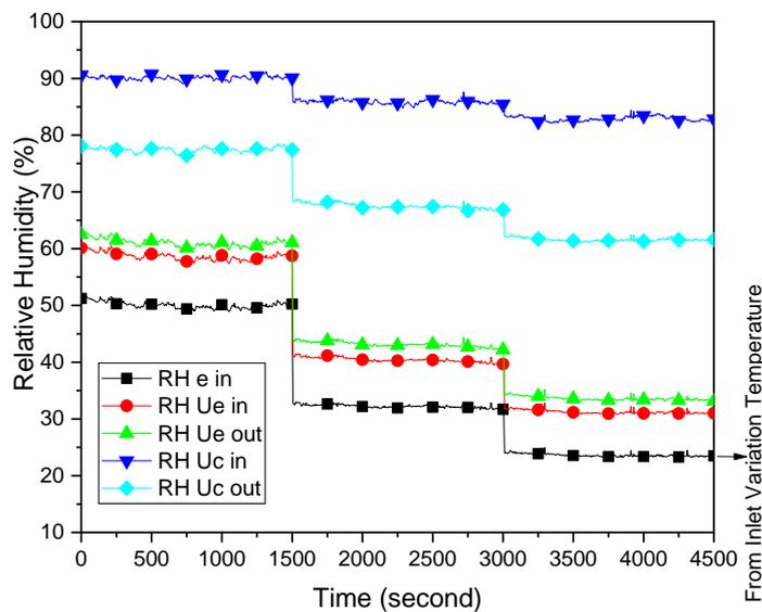
**Figure 5. The relative humidity of two-row U-shaped heat pipe with inlet air velocity of 2.5 m/s**
