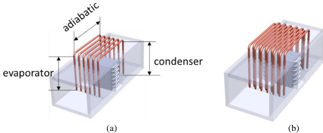
**Figure 1. (a) U-shaped Heat Pipe 1 Row; (b) U-shaped Heat Pipe 2 Row in a staggered configuration**
