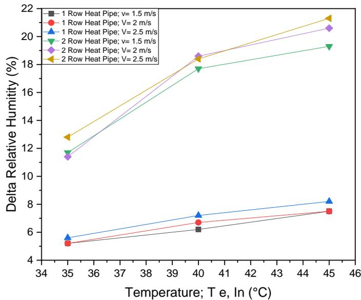
Figure 7. The difference of Relative Humidity in the condenser section of the U-shaped Heat Pipe
