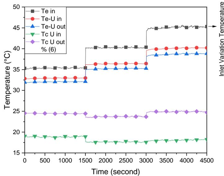
**Figure 4. The temperature profile of two-row U-shaped heat pipe with inlet air velocity of 2.5 m/s**
