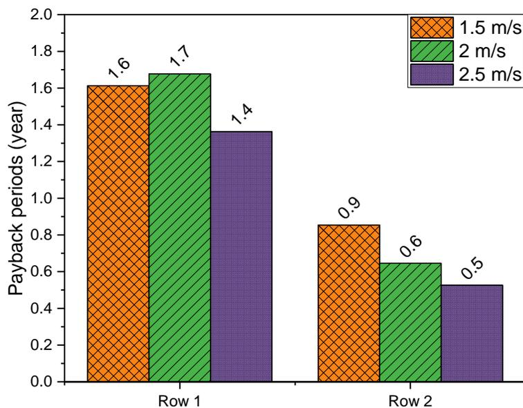
Figure 9. The Payback Periods of U-shaped Heat Pipe
