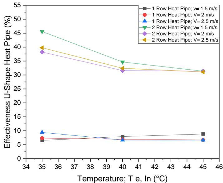
Figure 6. The effectiveness of the U-shaped Heat Pipe
