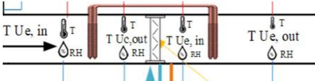
**Figure 3. Position of Temperature and RH sensor**
