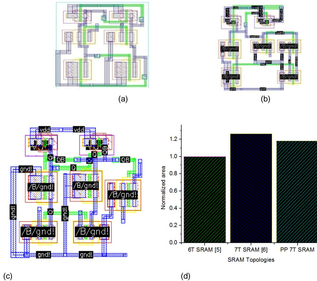
Figure.11 (a) Layout of Conv. 6T SRAM[5] (b) Layout of 7T SRAM [6], (c) Layout of PP 7T SRAM,(d) Normalized area of SRAM Topologies.
