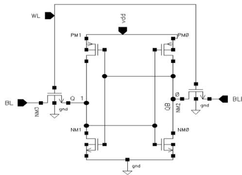
Fig.1: Standard 6T SRAM Cell [5]
