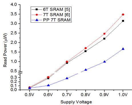
Figure 7: Read Power of SRAM topologies
