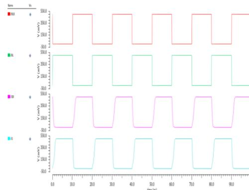
Figure 4: Write Waveform of PP 7T SRAM
