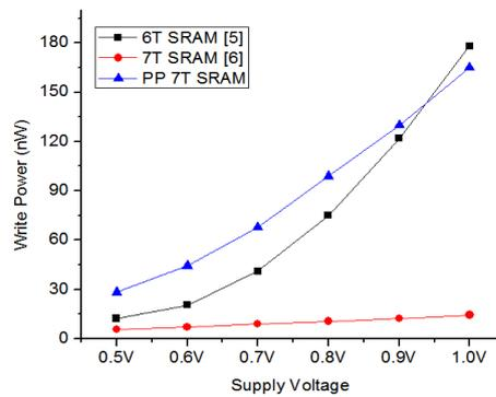
Figure 8: Write Power of SRAM topologies
