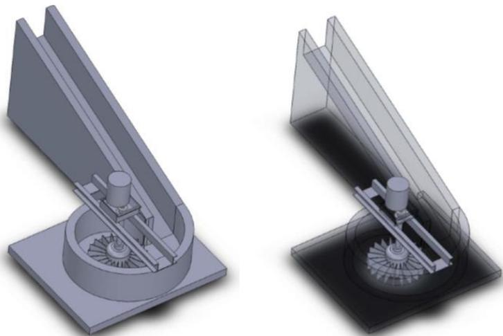
**Figure 3. Vortex Type Low Head Turbine Concept**
