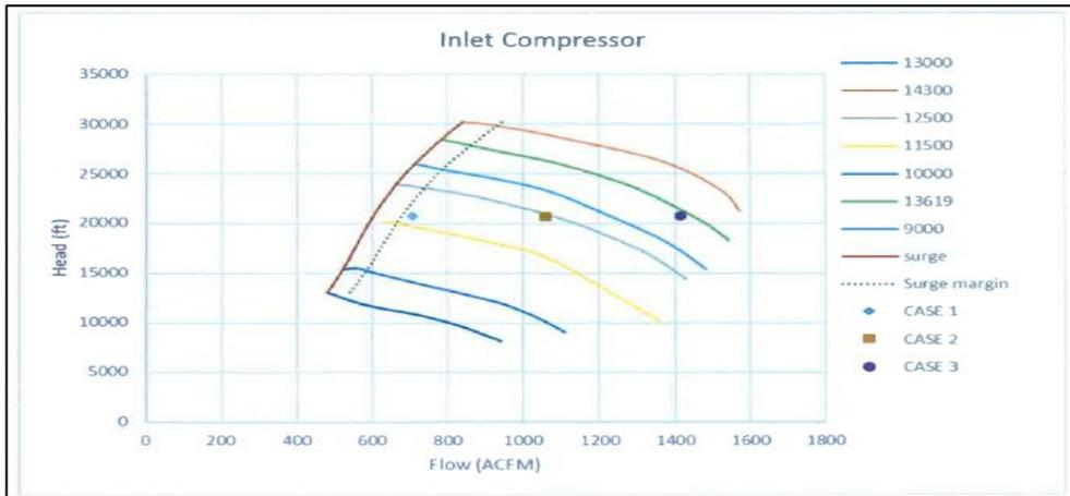
Figure 4. Compressor performances for Inlet Gas Rate
