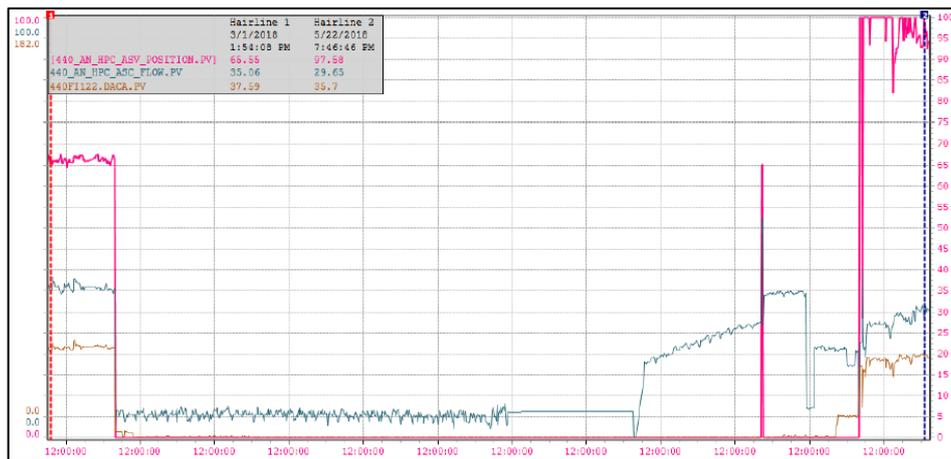
Figure 7. Anti-surge control valve position after restaged
