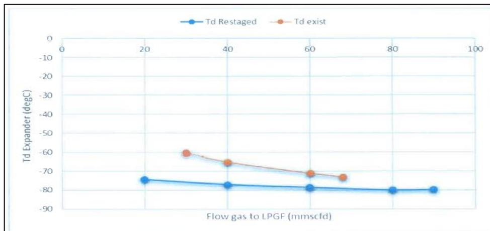
Figure 2. Turbo expander discharge temperature comparison
