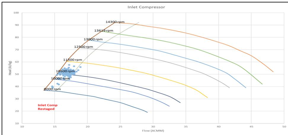
Figure 6. Inlet Compressor Performance Curve
