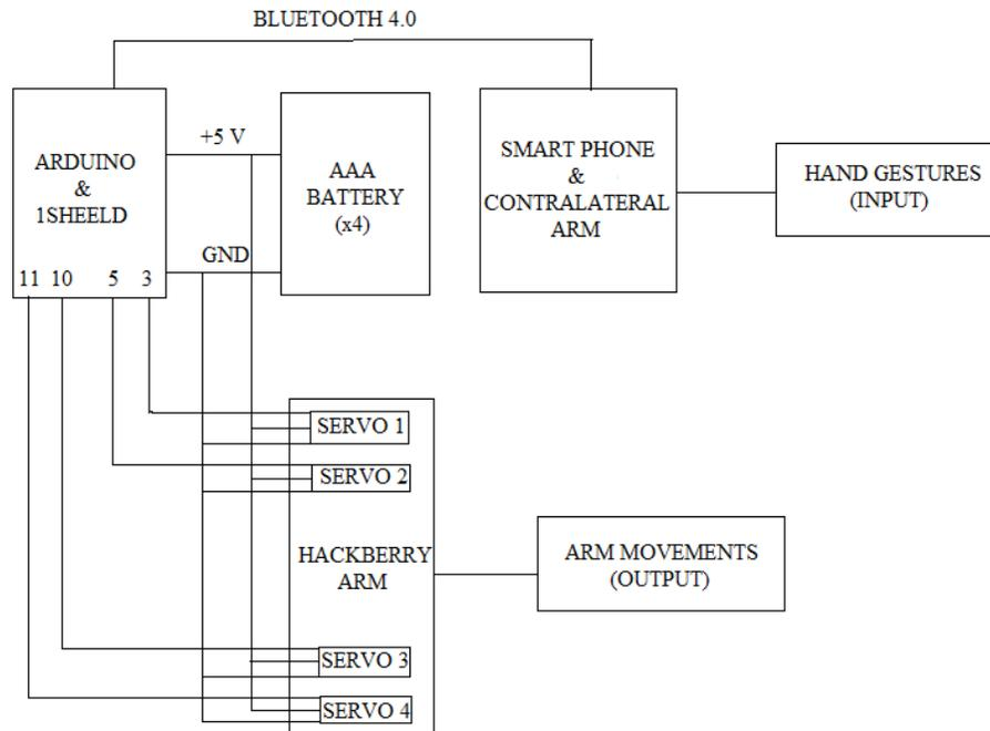
**Fig. 2** Circuit Diagram
