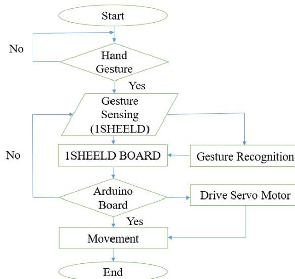
**Fig. 1** Flow Diagram
