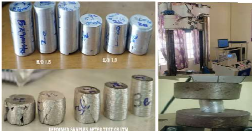
Fig 1.2 Machined Samples of aspect ratio 1.0 & 1.5 & Tested on UTM
