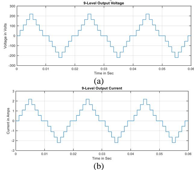
**Figure 1 Voltage and Current Output waveforms of 9-Level Inverter with R-Load**
