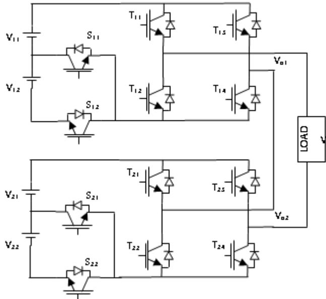
Figure 2 Circuit Diagram of Symmetrical 9-Level Modified CHBMLI
