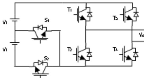
Figure 1 Generalized Basic Circuit for Cascaded Modified H-Bridge inverter
