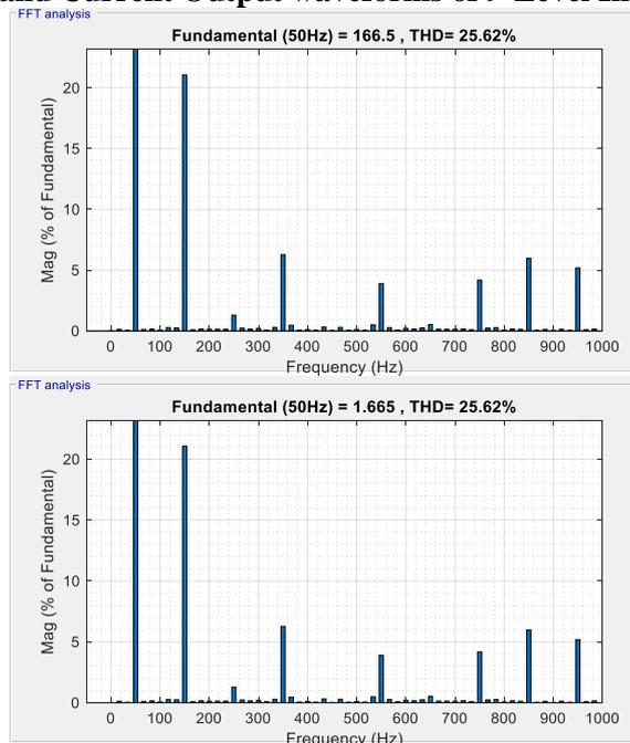
**Figure 2 Harmonic Spectra of Nine-Level Voltage and Current Output with R-Load**
