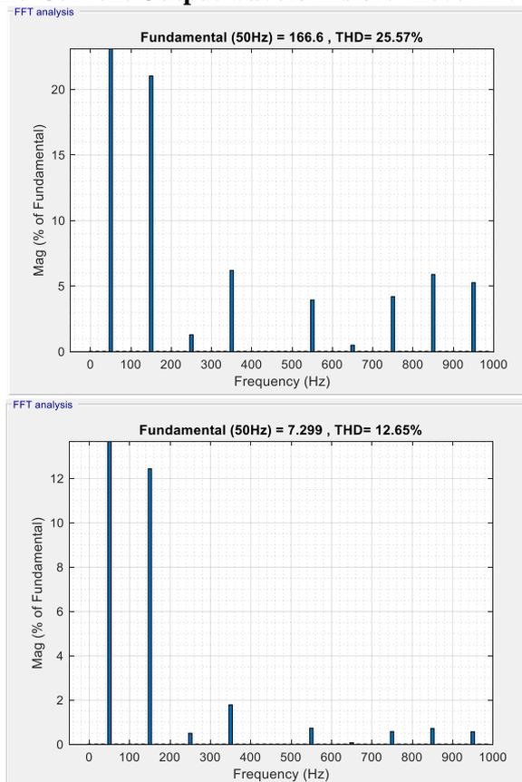
**Figure 4 Harmonic Spectra of 9-Level Voltage and Current Output with RL-Load**
