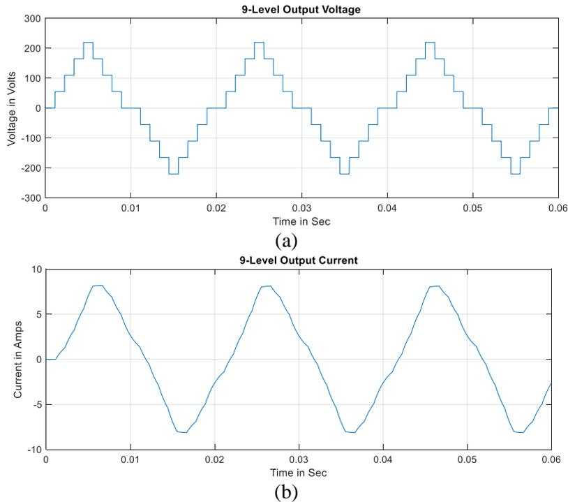
**Figure 3 Voltage and Current Output waveforms of 9-Level Inverter with RL-Load**
