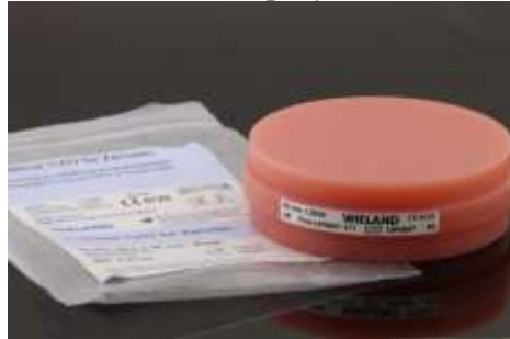
Fig1: Heat cure acrylic specimens
