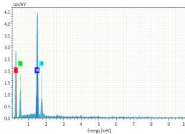
Fig.2 (e) EDS Analysis of hybrid composite coatings
