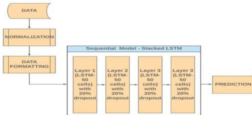
Fig. 7: The architecture of the proposed prediction system
