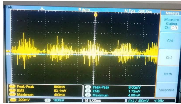
Figure 4.2: PD pattern for stress level of 1.4 times the inception. Input voltage (4.06Kv).
