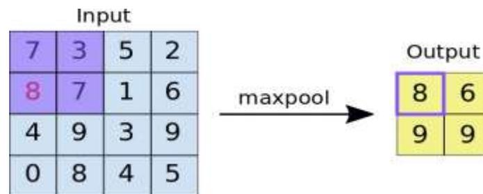
**Figure.4.** Example of Max Pooling
