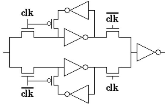
**Fig 1: Double Edge Triggered FlipFlop**
