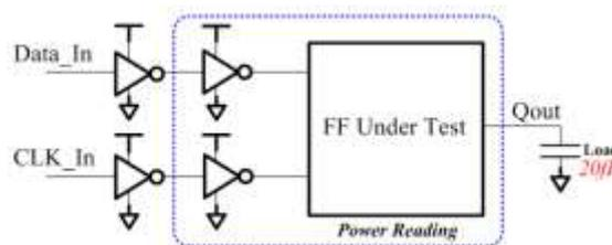
**Fig 2: Model setup for FF simulations**
