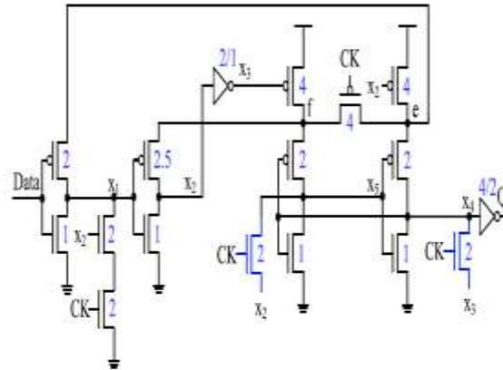
**Fig 2: Low paper 19T True Single Phase Clocking Flip Flop using Master-Slave.**
