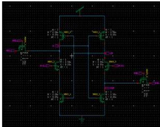
Fig. 4. Schematic of proposed 8T SRAM bitcell
