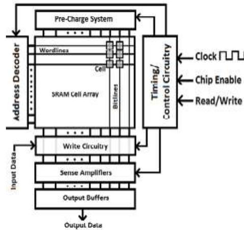
Fig. 3. Block Diagram of SRAM memory array.
