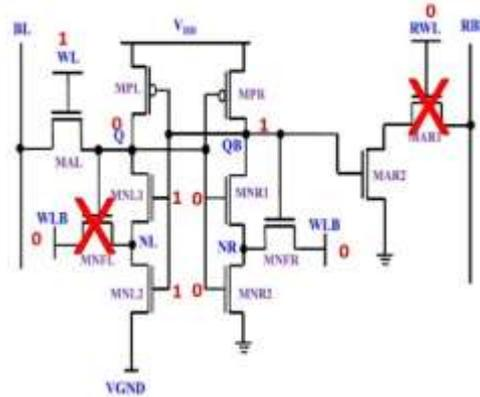
Fig. 2(a). 8T SRAM Cell write operation
