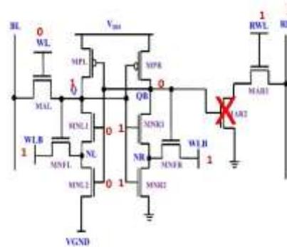
Fig. 1(a).8T SRAM Cell read operation
